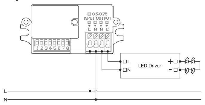
The sensor is allowed to be connected to one load only. The sensor may be damaged if connecting more than one load.
