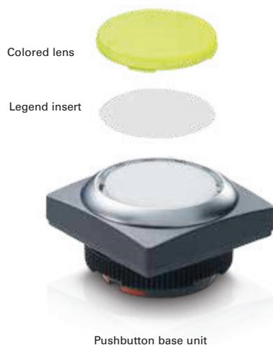
→ The RAFIX 22 FS+ FLEXLAB pushbutton allows individual control component labeling. A DIN A4 label sheet with pre-cut labels which fits in all customary office printers is available for this option. After the legend inserts are printed, the labels can be detached from the sheet and inserted into the colored lens using the fine stop tabs.
